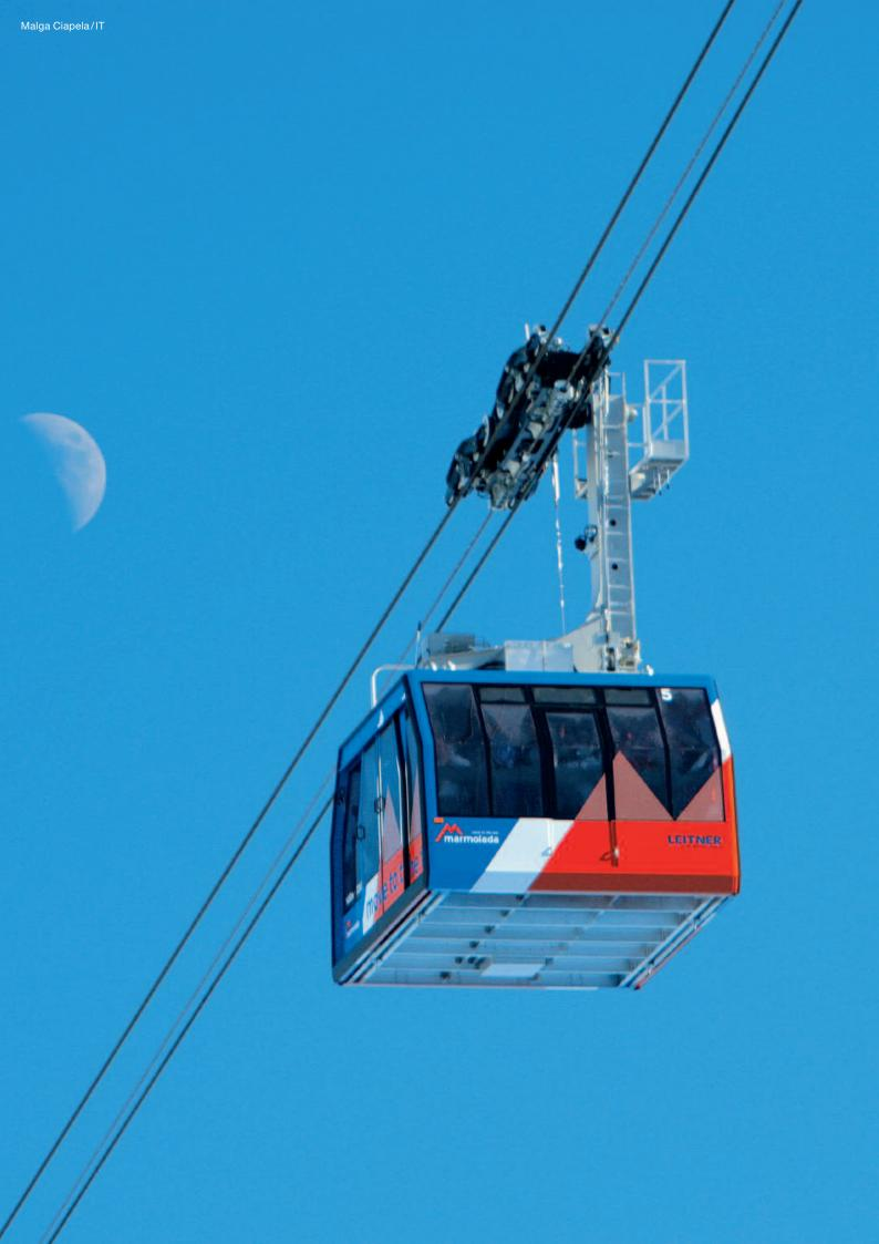
**AERIAL TRAMWAYS** are an attractive modern ropeway system that is ideal for extremely steep terrain, high levels of availability, good stability in wind, and outstanding operating reliability and safety. Aerial tramways have one or two carriers running to and fro either on one carrying hauling rope or on one or two track ropes, with a haul rope providing the traction.
